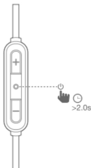
2. If connecting for the first time, the headphone will enter pairing mode automatically after it is powered on.
